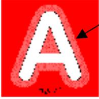
Shadowing is a "halo" effect that frequently occurs around the engraved character when the depth nose is used. It's one of the more common problems faced by engravers, but once the specific cause is identified it's usually easy to correct.
